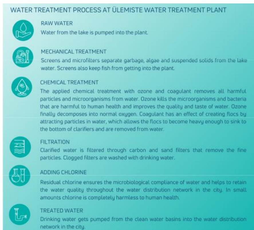
Figure 3: Description of water treatment process at Ülemiste Water Treatment Plant
