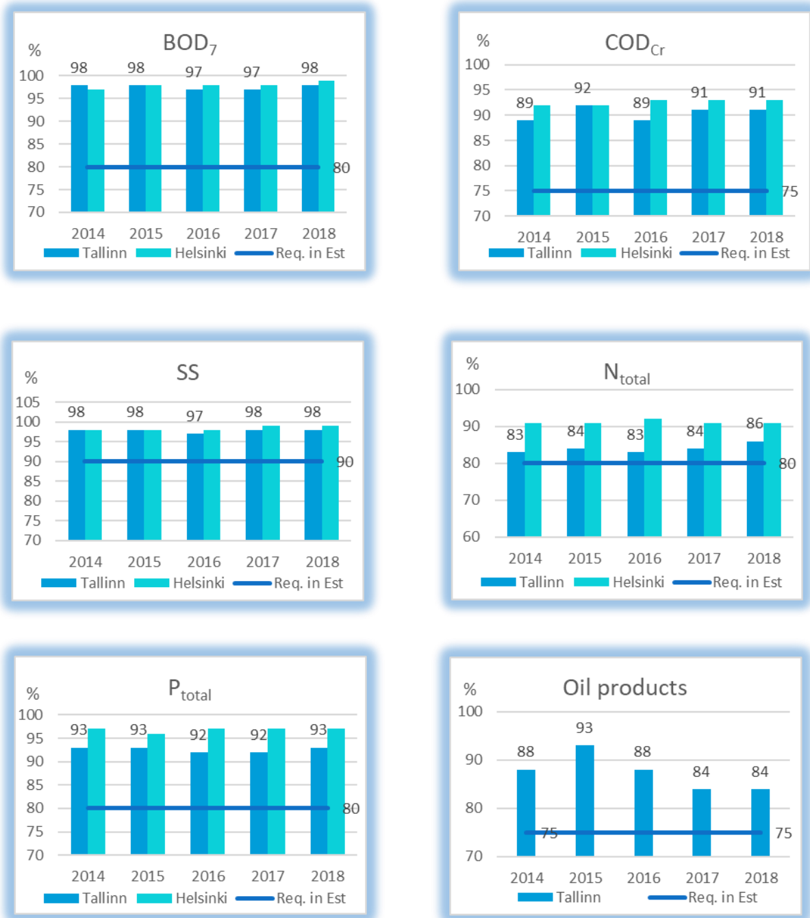
Chart 4: Wastewater treatment plant's treatment efficiency in 2014-2018, compared to regulatory minimum requirements and results of Helsinki HSY, %
