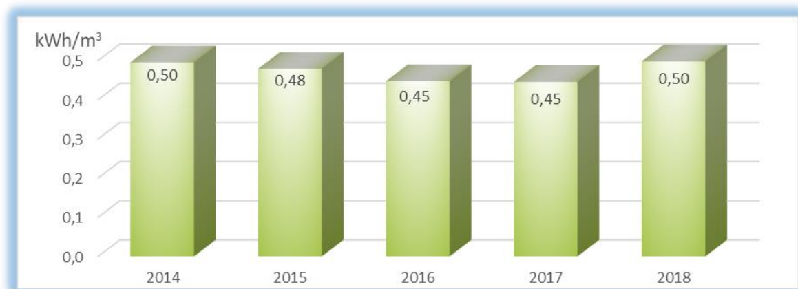
Chart 8: Electricity consumption per unit produced at wastewater treatment plant in 2014-2018, kWh/m 3
